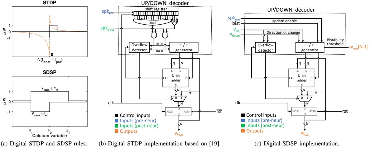
Fig. 1: Illustration of the STDP and SDSP learning rules together with their minimal N-bit implementations using clocked digital circuits.
