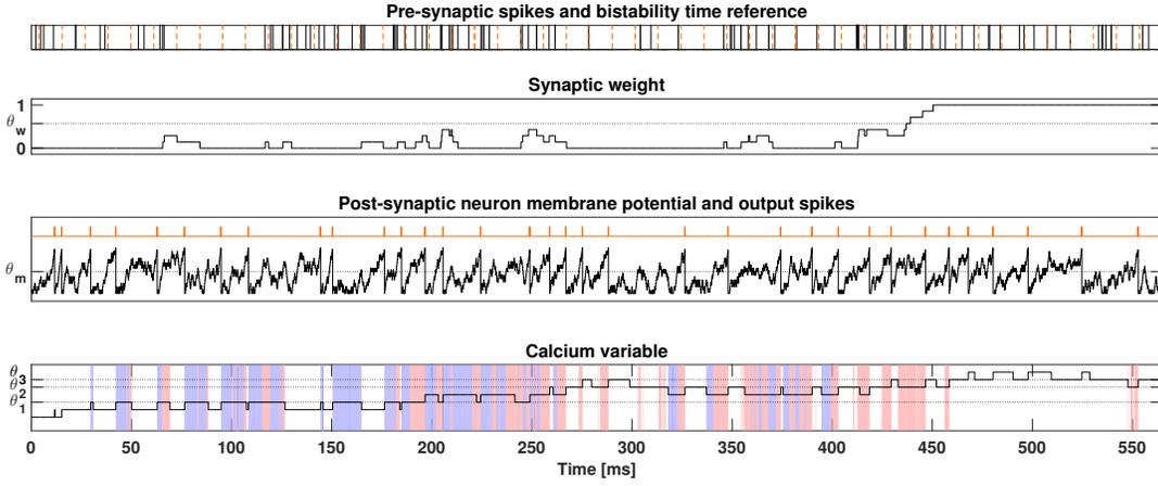
Fig. 4: Post-layout simulation of the proposed asynchronous SDSP-based synapse. The bistability `bist` reference trigger is shown as dotted orange lines next to the pre-synaptic spikes. The SDSP conditions for potentiation ( $v_{up}$ ) and depression ( $v_{down}$ ) from the post-synaptic neuron are shown next to the Calcium variable in red and blue, respectively. Non-colored parts of the Calcium concentration are associated with stop-learning conditions.
