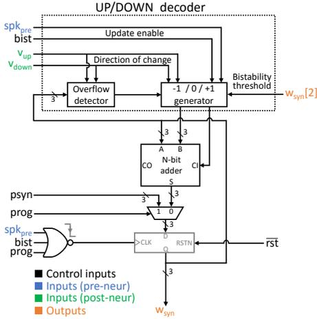
Fig. 3: Proposed SDSP-based 3-bit asynchronous programmable synapse.
